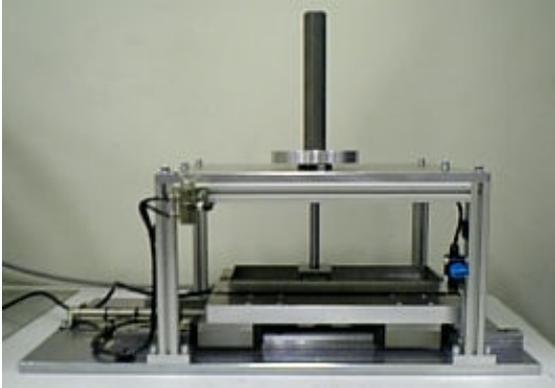
Fig.2 Experimental apparatus measuring the frictional coefficient of rubber sample with respect to ice surface.
