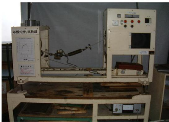
Fig.3 Testing machine to estimate CSR index for shoe soles
