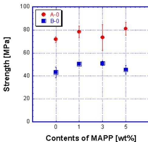
Fig 7(a) Flexural strength changes after humidity conditioning.
