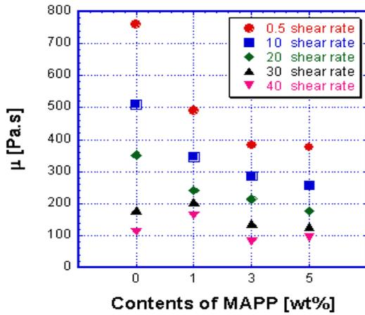
Fig. 2 Viscosity vs contents of MAPP at various shear rate
