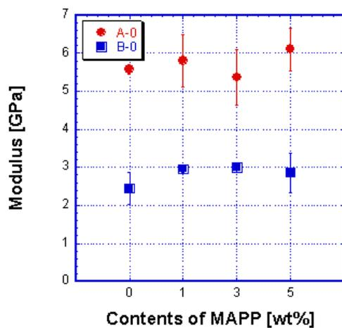
Fig 7(b) Flexural moduli changes after humidity conditioning.
