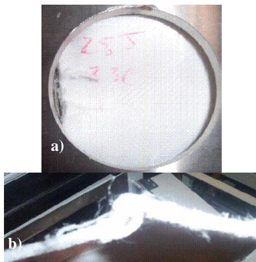
**Figure 8:** Bending caused by 25J impact on untreated samples; **a)** top view, **b)** side view
