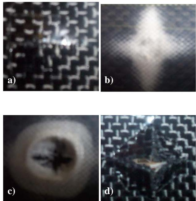
**Figure 9:** Damage types: **a)** back surface cracking, **b)** bending/plastic deformation, **c)** delamination, **d)** total penetration.
