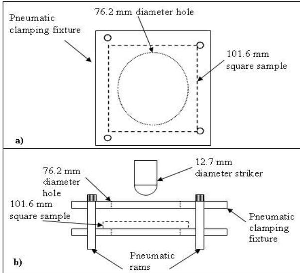
**Figure 2:** Pneumatic clamping fixture, a) top view, b) side view
