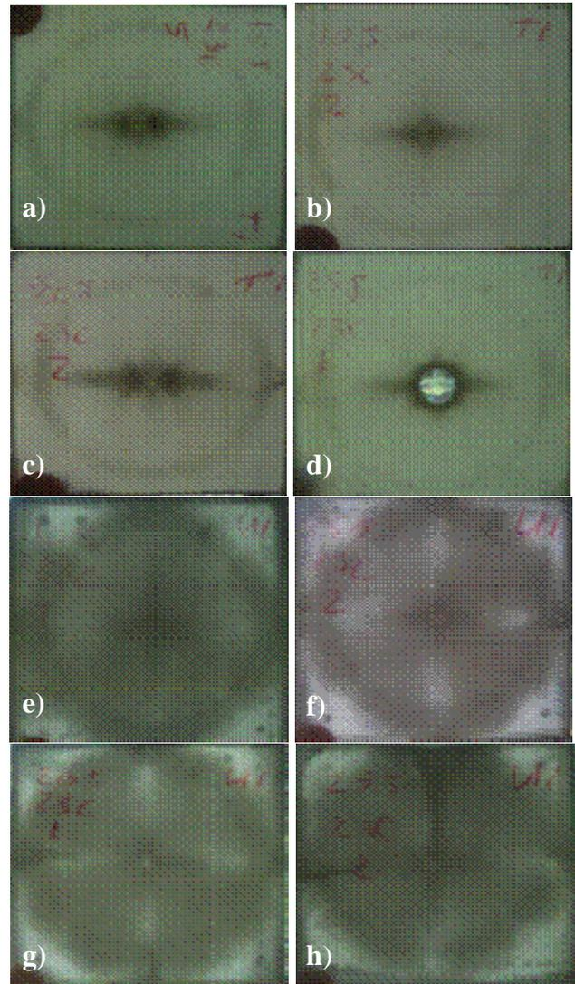
Figure 6: Delamination and damage of a) 10J treated, b) 15J treated, c) 20J treated, d) 25J treated, e) 10J untreated, f) 15J untreated, g) 20J untreated, and h) 25J untreated
