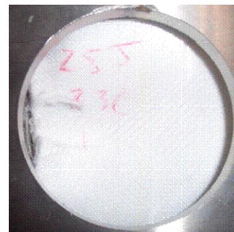
**Figure 4:** Untreated sample pressed into the clamping fixture.
