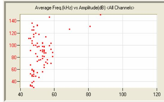
Fig. 7b. Freq (kHz) vs. Amplitude (dBAE) for GF/RC at  $-60^\circ\text{degC}$
