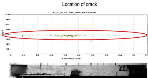
Fig. 13. 1-D Damage Location plot for CF/RC at 90% load and RT
