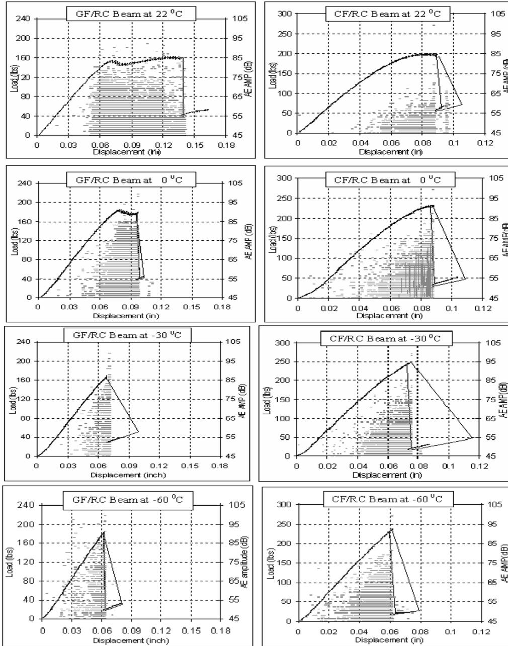
Fig. 4. Load (lb) vs Displacement (m) curves with superposed AE amplitudes (dBAE) vs Time (sec) curves for GF/RC (left) and CF/RC (right) for temperatures RT 22degC (top), 0 degC, -30 degC, and -60 degC (bottom).
