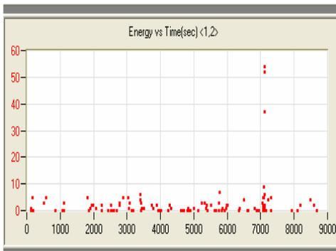
Fig. 7a. Energy ( $\mu\text{J}$ ) vs. Time (sec) for GF/RC at  $-60^\circ\text{degC}$
