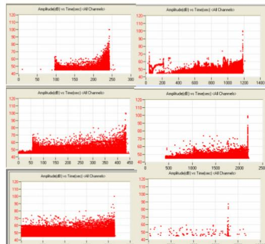
Fig. 12 Characteristic Amplitude (dBAE) vs, Time (sec), plots for RT, 22degC (top), -30 degC (middle), and -60 degC (bottom), for CF/RC (left) and GF/RC (right)
