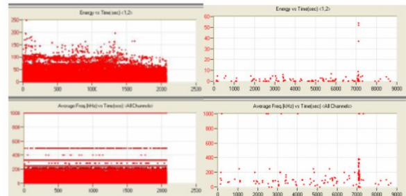
Fig. 11 Characteristic Energy ( $\mu\text{J}$ ) vs, Time (sec), top and Freq (kHz) vs Time (sec), bottom, responses of CF/RC (left) and GF/RC (right).
