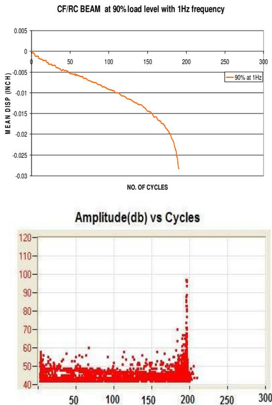
Fig. 3. Typical Disp-Cycles curve with attached AE amplitudes (RT CF/RC)
