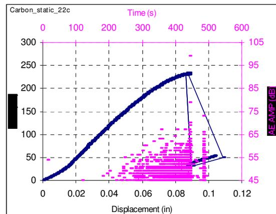
Fig. 2. Typical Load-Displacement curve with superposed AE amplitudes (RT GF/RC)
