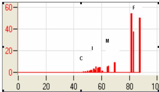
Fig. 6. Energy ( $\mu\text{J}$ ) vs Amplitude (dBAE) for GF/RC at  $-60^\circ\text{C}$
