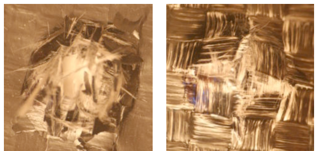
Fig. 6. Damaged area for dynamic / static perforation
