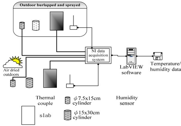
Fig. 6. Experimental set-up for strength growth monitoring of a concrete slab.
