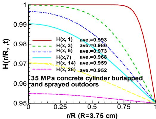
Fig. 13. The humidity profile of a concrete cylinder with outdoor burlapped and sprayed
