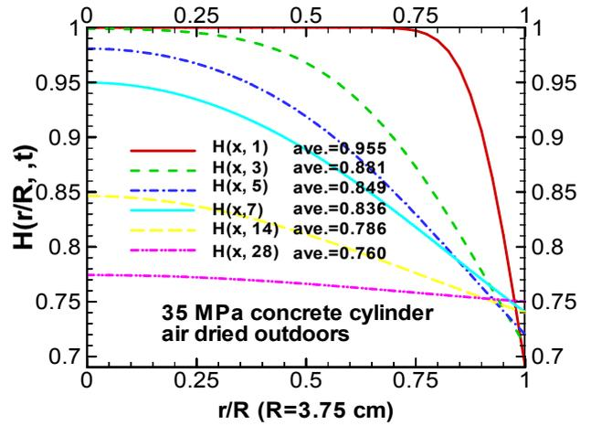
Fig. 14. The humidity profile of a concrete cylinder air dried outdoors
