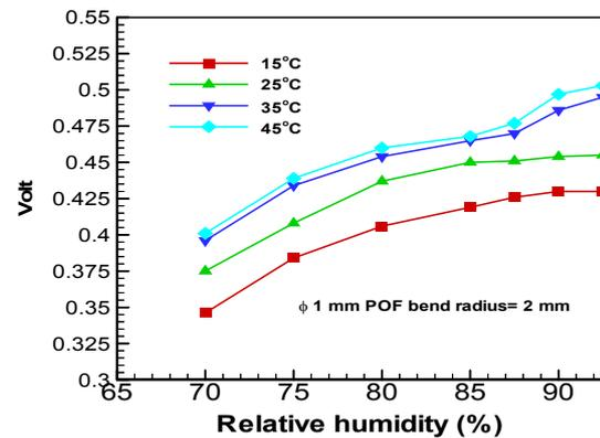
Fig. 2. The POF humidity response at different temperature and humidity
