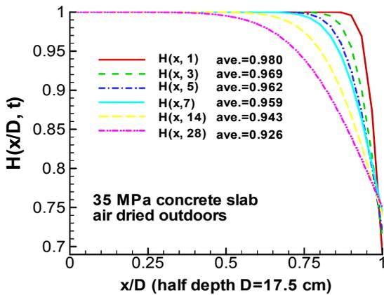
Fig. 12. The humidity profile of a concrete slab air dried outdoors
