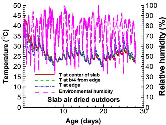
Fig. 8. The temperature and humidity of an outdoor air dried concrete slab
