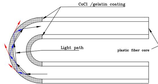
Fig. 1. The coating detail of a POF humidity
