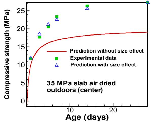
Fig. 9. Strength growth prediction of a concrete slab
