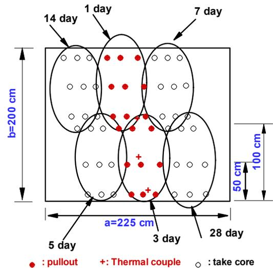
Fig. 5. Take-core, pullout and thermal couple positions of a concrete slab
