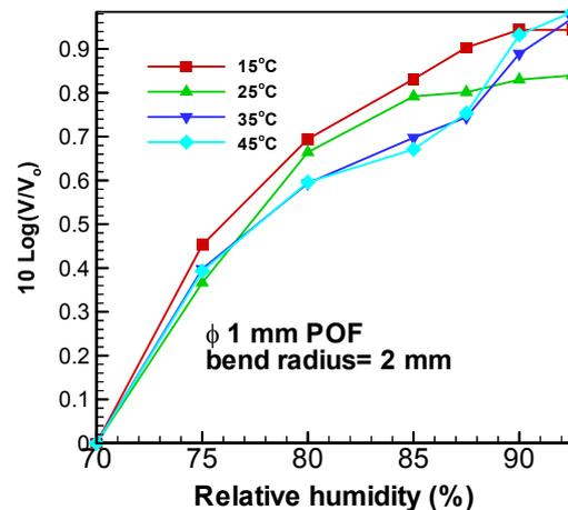
Fig. 3. The power loss of POF sensor at different temperature
