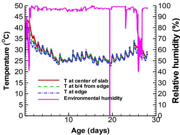
Fig. 7. The temperature and humidity of an outdoor burlapped and water sprayed concrete slab
