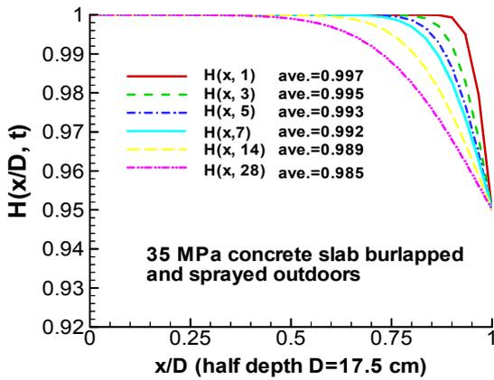
Fig. 11. The humidity profile of a concrete slab with outdoor burlapped and sprayed.
