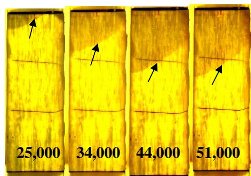
Fig. 8. Schematic of GFRP-GFRP bonded joint showing the disbond growth from the higher wavelength end of CFBG at various increasing fatigue cycles.
