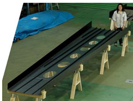
Fig. 10 Skin-Stringer integral molded 6m wing lower panel
