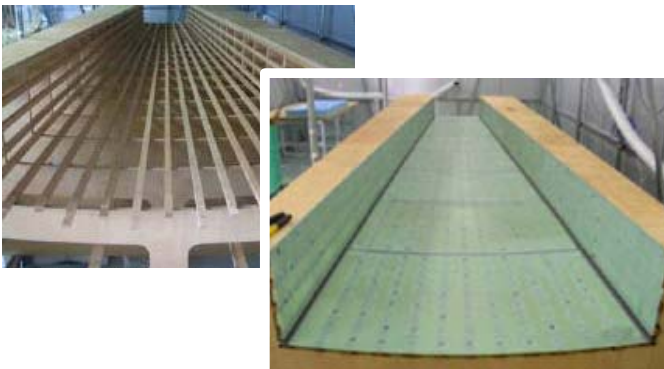
Fig.8 Wooden forming tool (lamination and curing)
