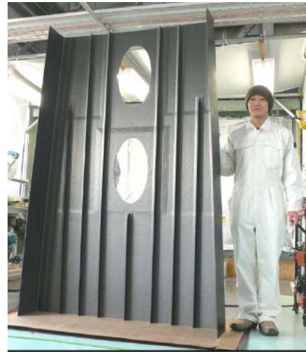
Fig.7 The general view after completing the manufacture of 2m stiffened panel
