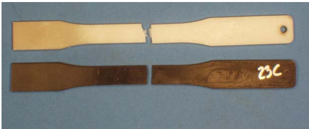
Fig. 3 Optical Images of Specimens Post Tensile Testing: Above, SC-15 Neat and Below, 1.0 wt.% SiC/SC-15
