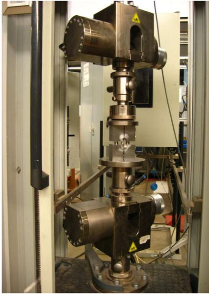
Fig. 2. Compression Test Set-up and the combined loading compression (CLC) test fixture.
