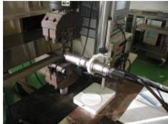
Fig. 2. In-situ observation of damage progress on the top surface during a tensile test.
