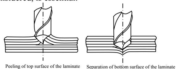
Fig.1. Drilling induced interlaminar delamination.
