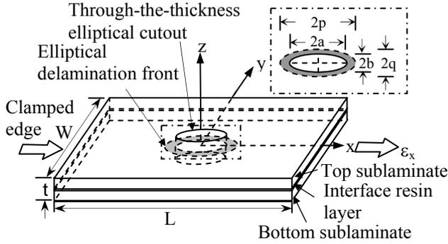
Fig. 2. Schematic of the laminate specimen with an elliptical interfacial delamination in the resin layer emanating from the edge of the elliptical cutout.
