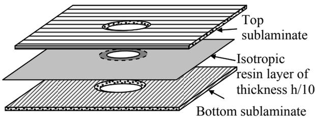
Fig. 3. Exploded view of the laminate specimen with an elliptical interfacial delamination in the resin layer emanating from the edge of the
