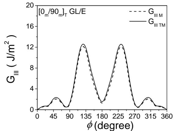
Fig.8.  $G_{III}$  distribution at 0/90 interface of  $[0_m/90_m]_T$  GL/E composite laminate.
