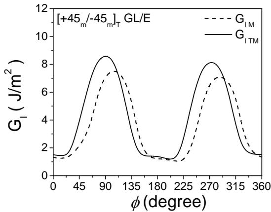
Fig.9.  $G_I$  distribution at +45/-45 interface of  $[+45_m/-45_m]_T$  GL/E composite laminate.
