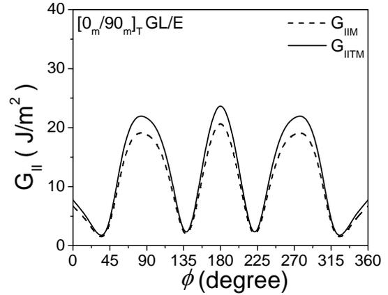
Fig.7.  $G_{II}$  distribution at 0/90 interface of  $[0_m/90_m]_T$  GL/E composite laminate.
