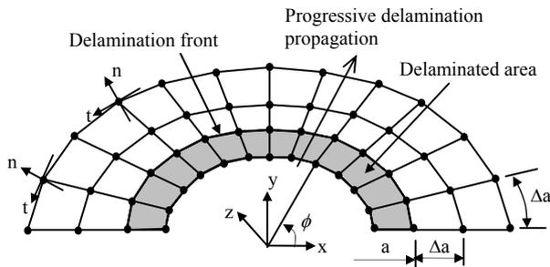
Fig.4. Interfacial elliptical delamination front
