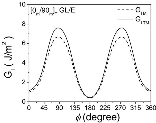
Fig.6.  $G_I$  distribution at 0/90 interface of  $[0_m/90_m]_T$  GL/E composite laminate.
