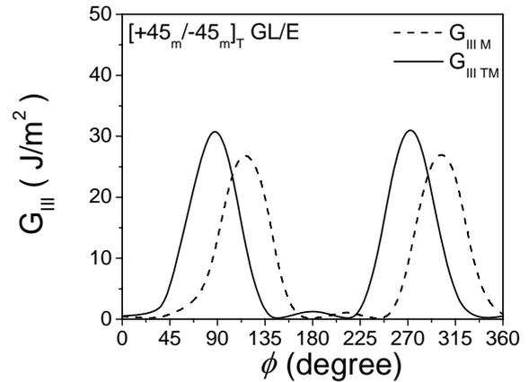
Fig.11.  $G_{III}$  distribution at +45/-45 interface of  $[+45_m/-45_m]_T$  GL/E composite laminate.
