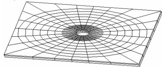
Fig. 5. Finite element meshing of the laminate specimen containing annular shaped elliptical delamination in the resin layer along at the interface along the edge of the central elliptical cutout.
