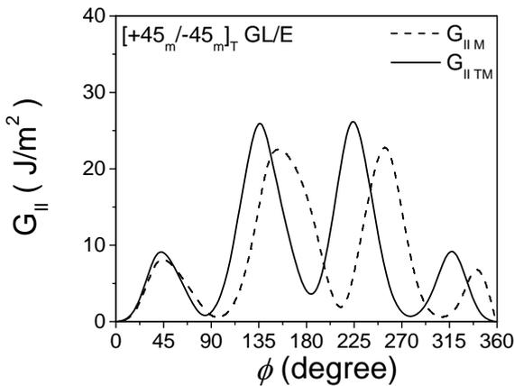
Fig.10.  $G_{II}$  distribution at +45/-45 interface of  $[+45_m/-45_m]_T$  GL/E composite laminate.
