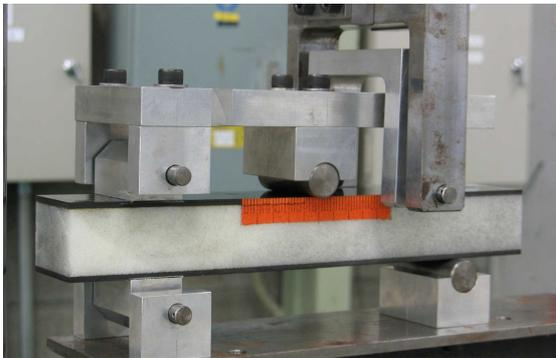
Fig.8 Specimen and loading device for mixed-mode type loading test
