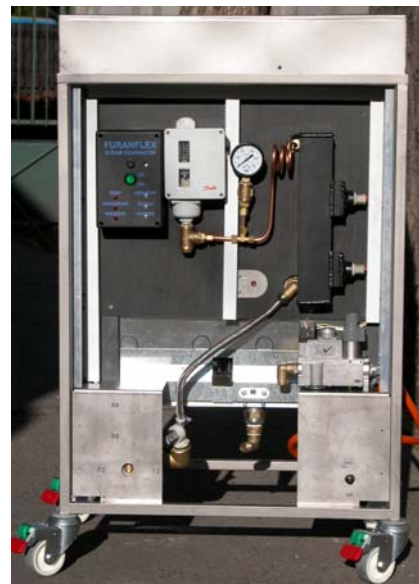
Fig. 13 FuranFlex® KNK 36 type steam generator
