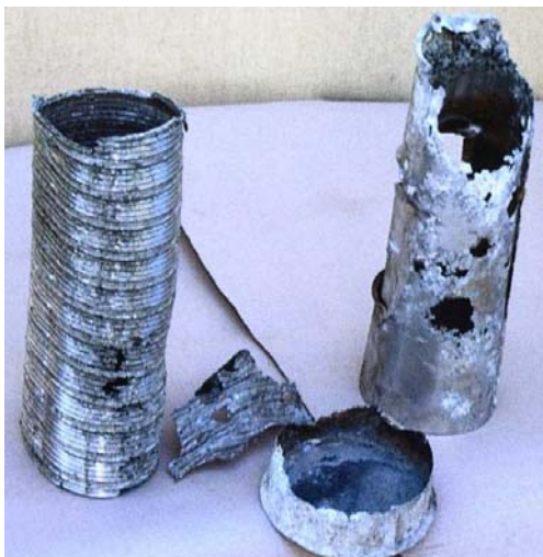
Fig. 2 Corroded aluminum chimney after 5 years of operation
