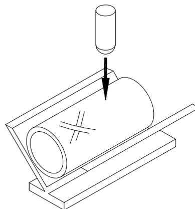
Figure 3. Tubular specimen's support for the impact tests
