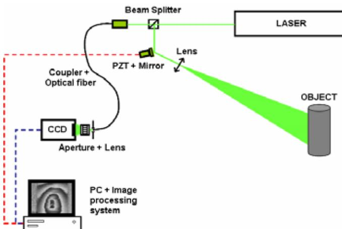
Figure 5. Schematic picture of the ESPI set-up
