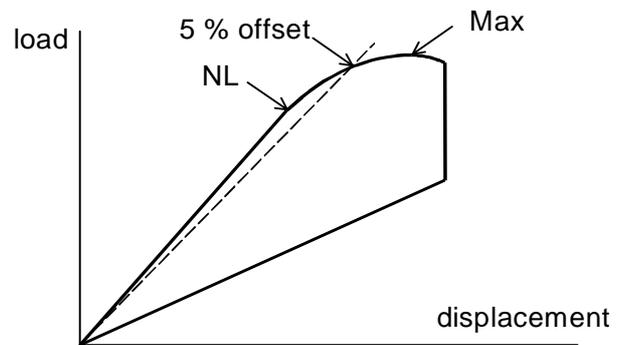
Figure 2 Used crack initiation criteria
