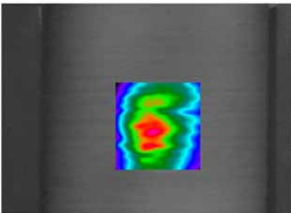
Figure 8. Defect zone after filtering
