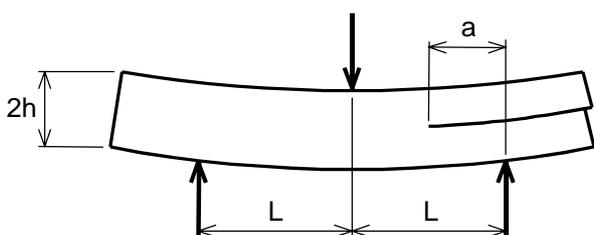
Figure1. Specimen's geometry for the ENF tests
