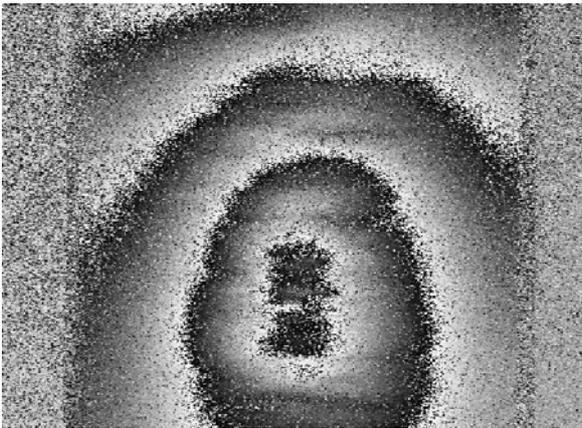
Figure 7. Phase map resulting from the captured raw fringe pattern
