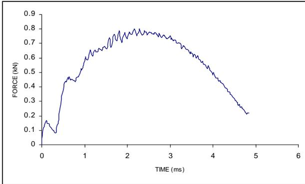
Figure 4. Force time chart from impact tests for a typical glass/polyester pipe
