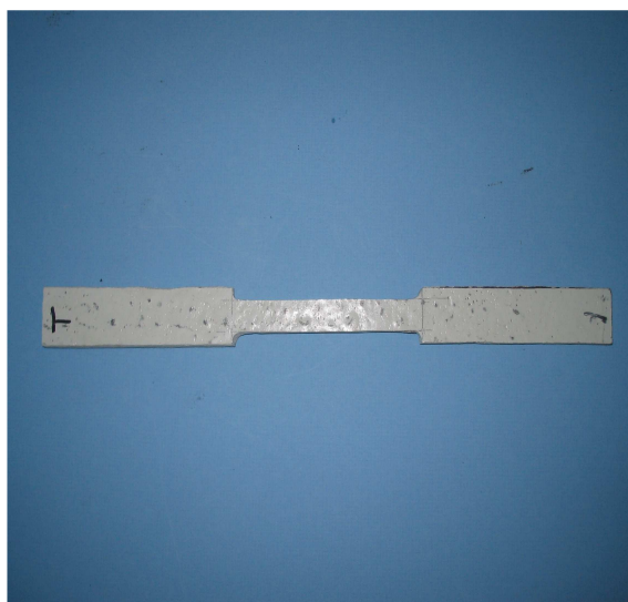
Fig. 3. Image of the tensile test specimen [1]
