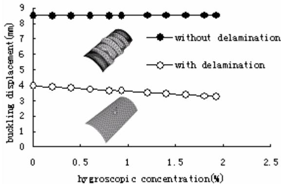
Fig. 5. Buckling loads vs hygroscopic concentration
