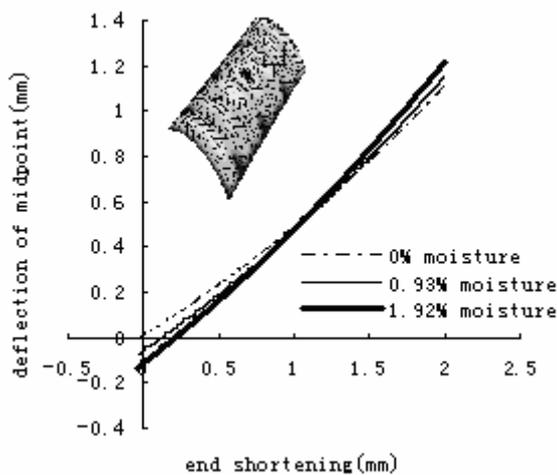
Fig. 6. Deflection of midpoint in the upper sub-plate vs end shortening
