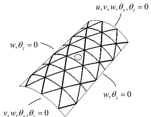
Fig. 4. Schematic of triangle AGS shell with a central circle delamination
