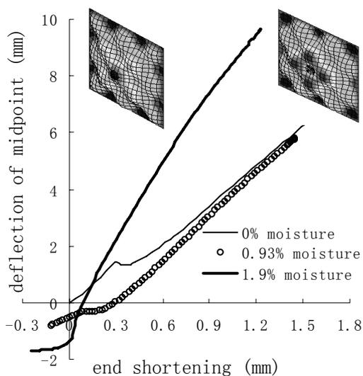
Fig. 3. Deflection of midpoint in the upper sub-laminates vs end shortening
