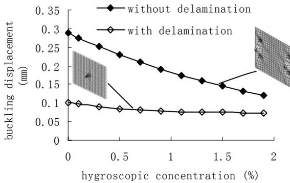
Fig. 2. Buckling loads vs hygroscopic concentration
