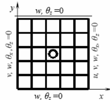
Fig. 1. Schematic of square orthogonal isogrid AGS plate with a central delamination
