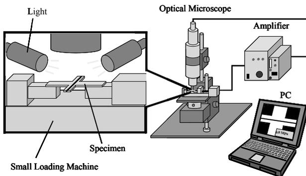
Fig.2 Schematic illustration of the observation system
