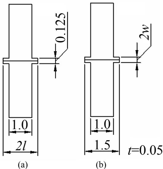
Fig.4 Schematics of FEM models to design specimen shape (a) analytical examination of  $2l$  and (b) analytical examination of  $2w$
