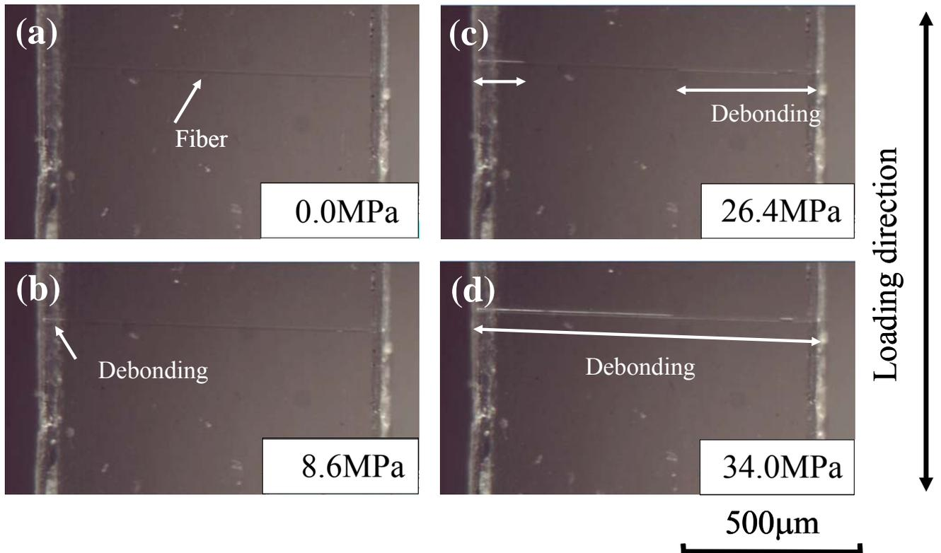
Fig.6 Debonding initiation and progress in a straight specimen
