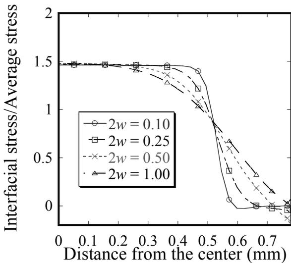
(b) Effect of  $2w$ Fig.5 Results of finite element analysis to design specimen shape. (a) Effect of  $2l$  and (b) Effect of  $2w$
