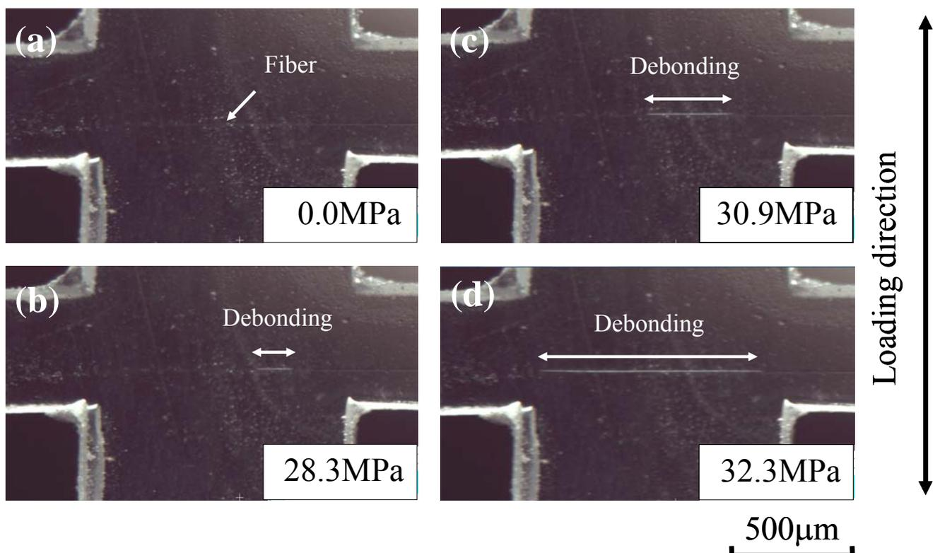
Fig.7 Debonding initiation and progress in a cruciform specimen
