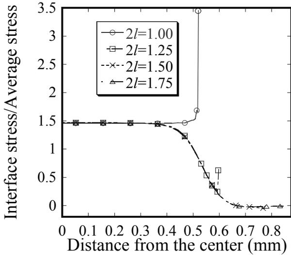
(a) Effect of  $2l$
