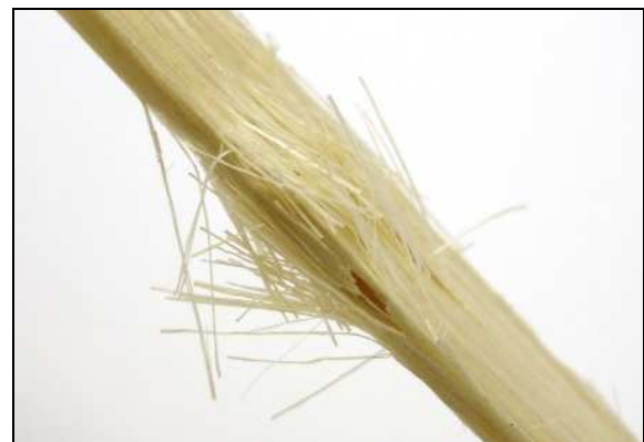
Fig. 10. Typical failure mode of an IFJ.
