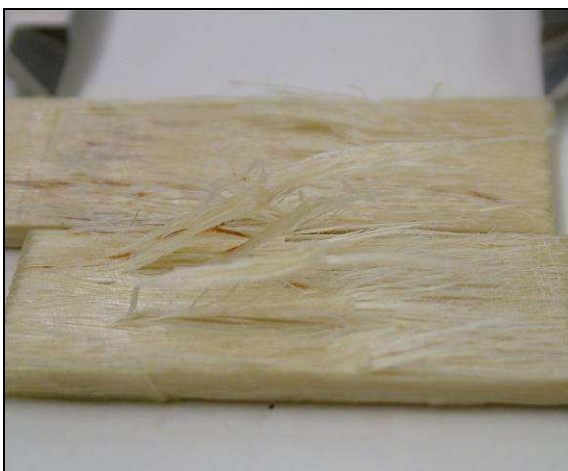
Fig. 8. Fibre-tear failure mode.
