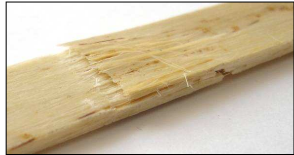
Fig. 13. Typical failure mode of an LFJ
