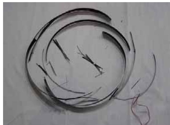
Fig.5. Fracture mode of CFRP in the impact test for the CFRP guarder belt
