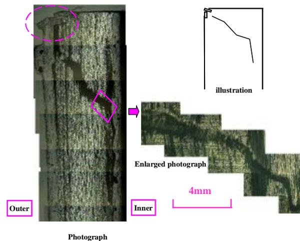
Fig.5. Cross section through the crush zone of UD carbon/polyester FRP tube crushed under R2 device during the initial load increasing stage.
