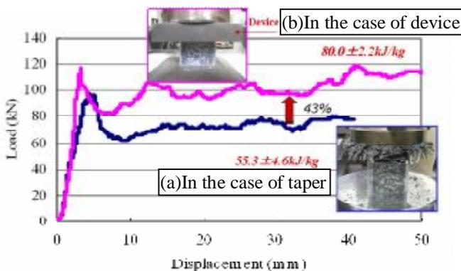
Fig.3. Test results of UD carbon/Polyester FRP tubes from the both compression modes i.e. (a) taper and (b) device.
