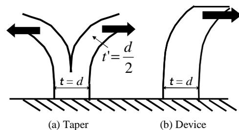
Fig.7. Crushing behavior (taper vs. device)
