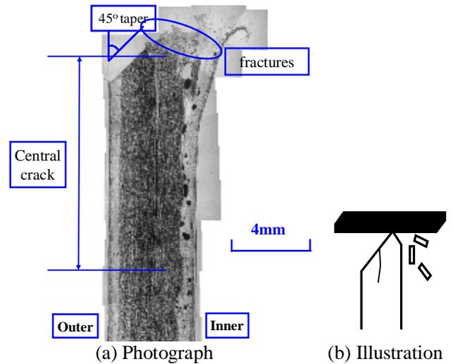
Fig.4. Cross section through the crush zone of UD carbon/polyester FRP tube with a taper during the initial load increasing stage.
