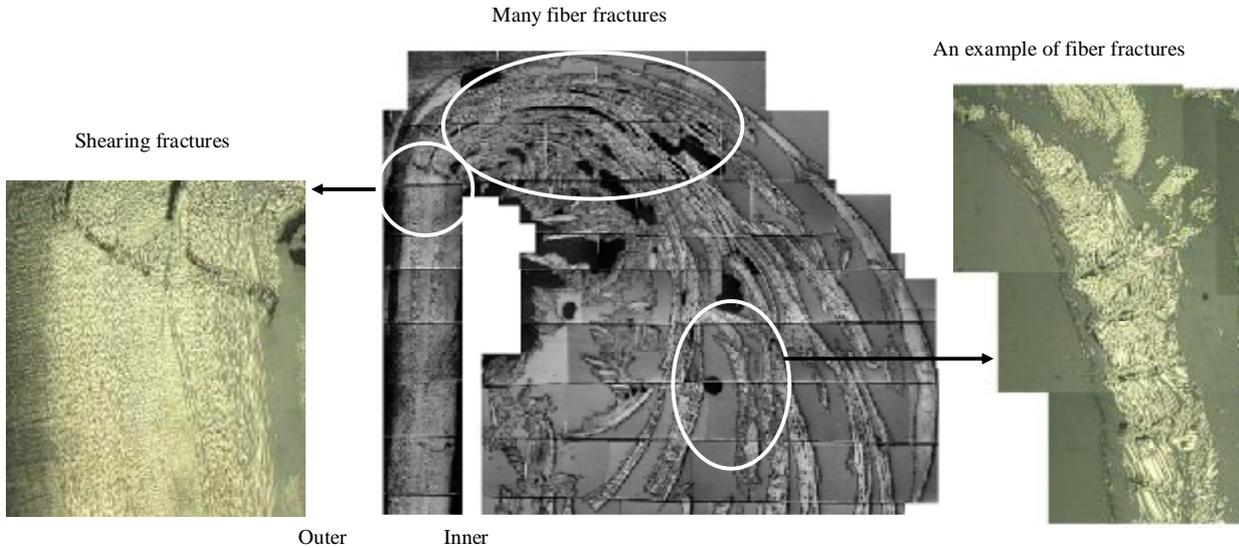
Fig.6. Observation results on the cross section through the crush zone of Carbon braided/epoxy FRP tube which crushed directly under the R3 device in the quasi-static compression test.
