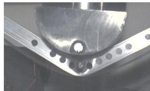
Fig.9 Breakage of Adhesive laminates (Specimen No.12)
