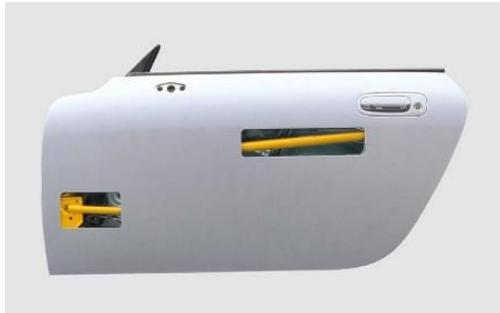
Fig.1 Door guard beam for side collision
