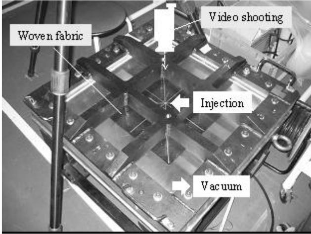
Fig. 6. Tool for radial flow test.
