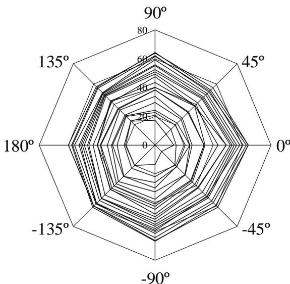
Fig. 7. Flow front radius during 21 sec (ID2). (Each contour line corresponds every sec.)
