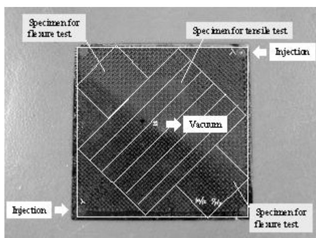
Fig. 5. Weld line and cut-pattern of specimens.
