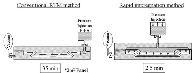
Fig. 4. Schematic of two resin injection methods.
