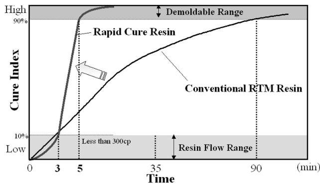
Fig. 3. Concept of the rapid cure resin.
