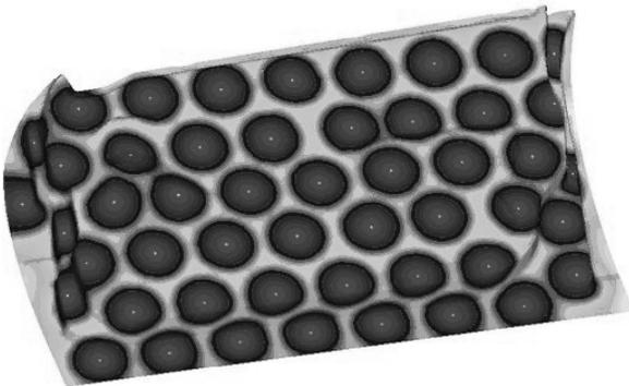
Fig. 11. Simulation result of multi-gate injection.
