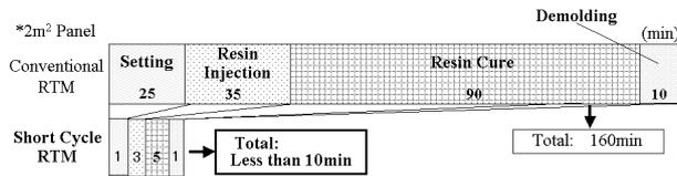
Fig. 2. Time apportionment of RTM molding process.
