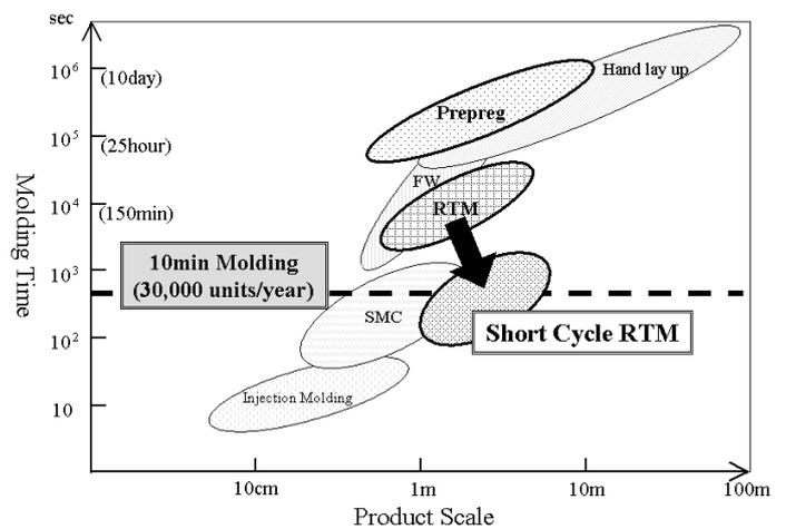
Fig. 1 Target of Short cycle RTM.
