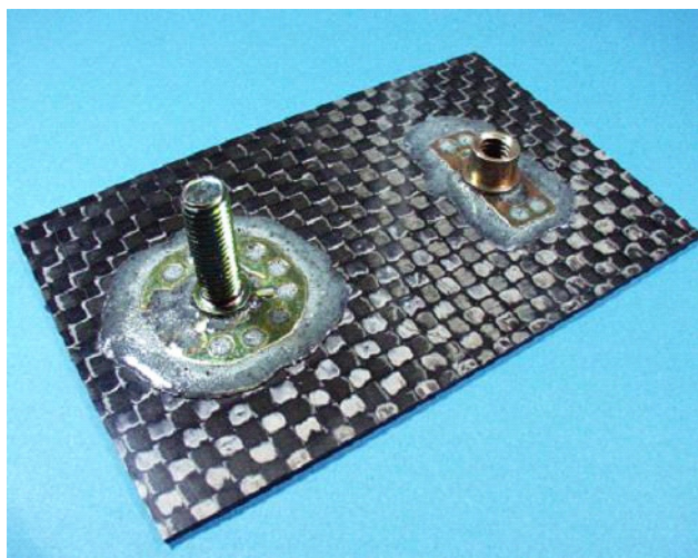
(a) Joints consisted of a CFRP and steel plates adhered with dismantlable adhesives (DGEBA (828) / DGEBA (1001) / GPI = 30 / 45 / 25 with 10 phr of CSR and 10 wt% of expandable graphite)
