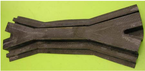
Fig. 10. Cross-beam demonstrator produced by vacuum infusion.
