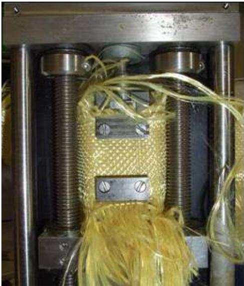
Fig.11. Tensile loading of the sample
