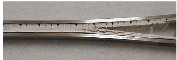
Fig. 5. S-2 glass 3WEAVE ® composite specimen after DCB testing
