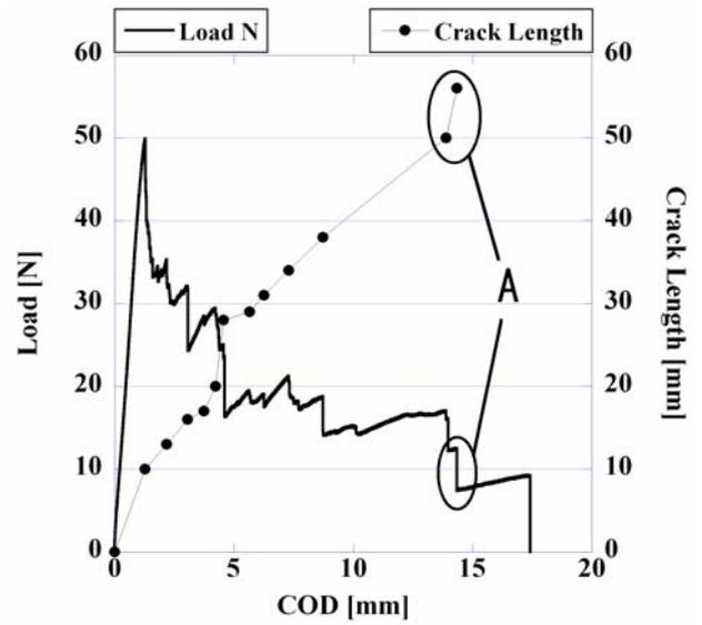
Fig. 8 Load-COD curves applied Zanchor
