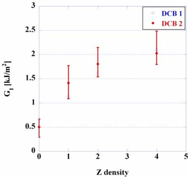
Fig. 7 Comparison  $G_I$ -Zanchor density between DCB Test 1 and 2
