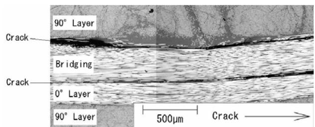
Fig. 10 Photograph of bridging fibers on side after DCB test
