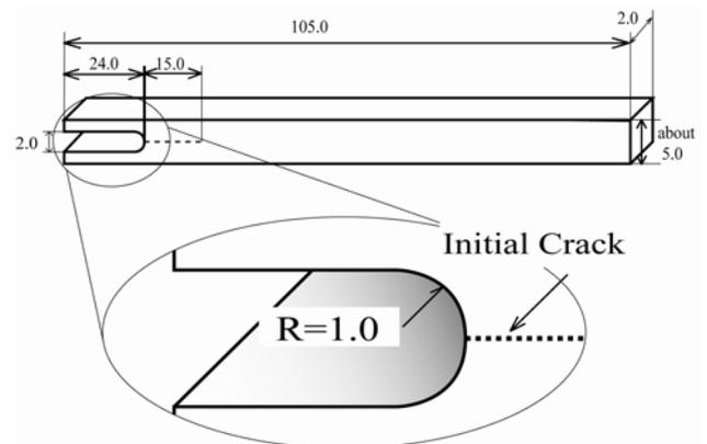
Fig. 6 Dimensions of DCB Test 2
