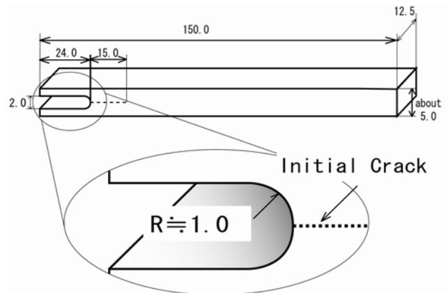
Fig. 2 Dimensions of DCB Test 1
