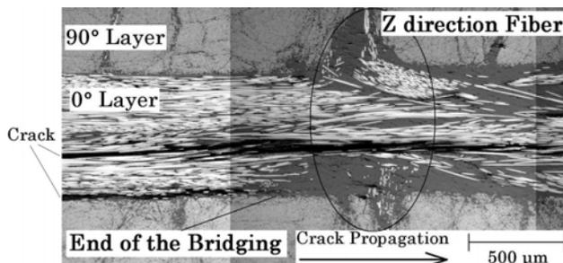
Fig. 12 Photograph of bridging fibers on ending point
