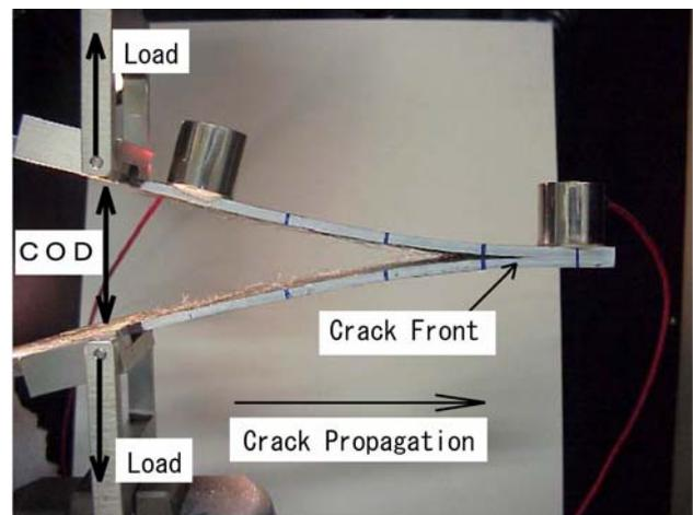
Fig. 3 Test setup of DCB Test 1
