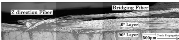
Fig. 11 Photograph of bridging fibers on starting point
