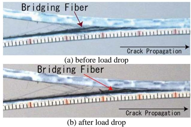
Fig. 9 Photograph on side before and after load drop
