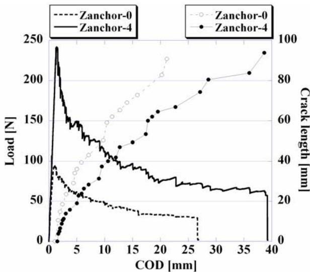
Fig. 4 Comparison Load-COD curves between Zanchor0 and Zanchor4
