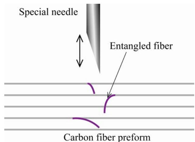
Fig. 1 Schematic of Zanchor
