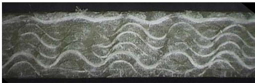
Fig.2 Cross-section of 3-D angle-interlock woven composites
