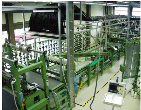
Fig. 1. Stitch bonding machine 14024 Karl Mayer Malimo
