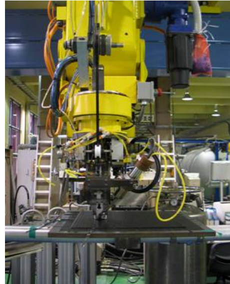
Fig. 2 Fiber placement system.
