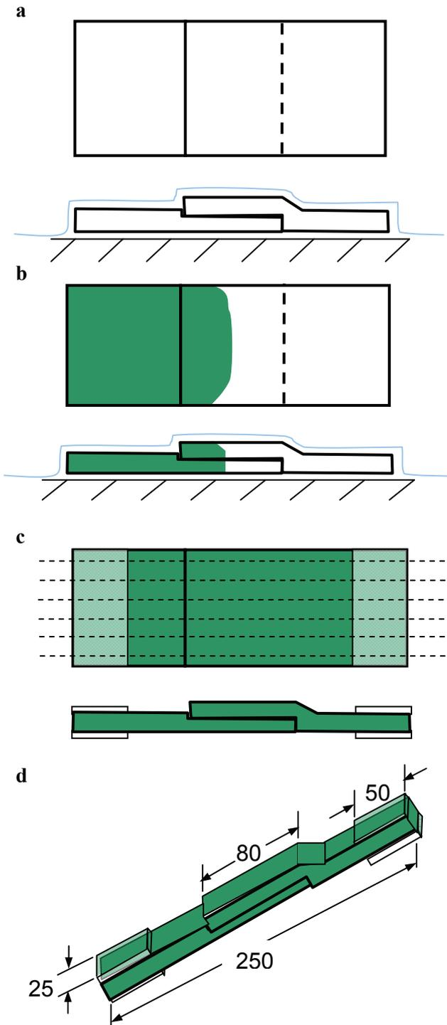
Fig. 5. Schematic of a step-by-step joint fabrication
