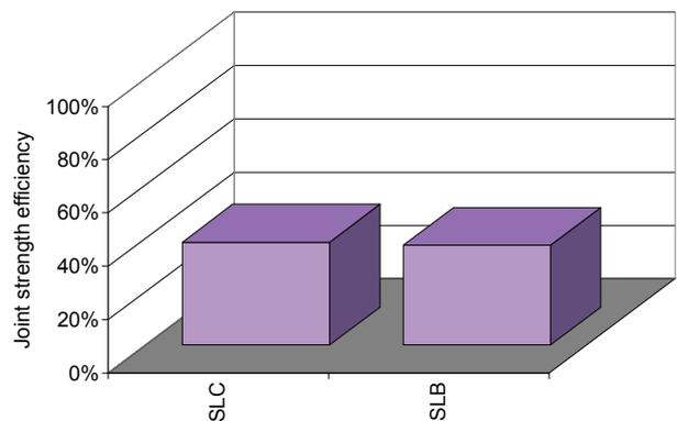
Fig. 9. JSE for co-cured (SLC) and bonded (SLB) single-lap joints
