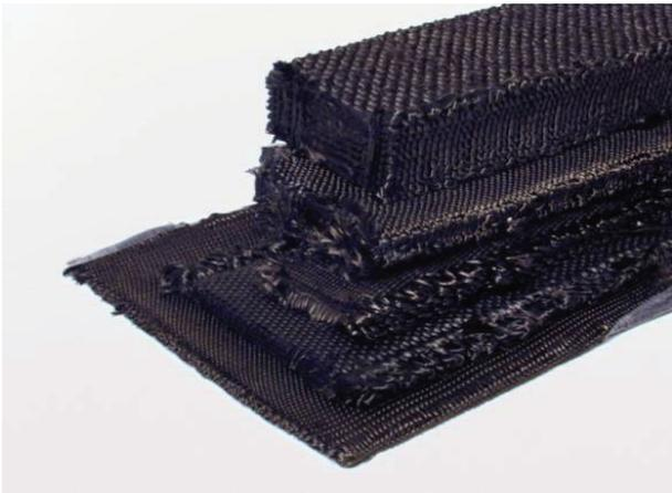
Fig. 2. Examples of 3WEAVE™ carbon preforms
