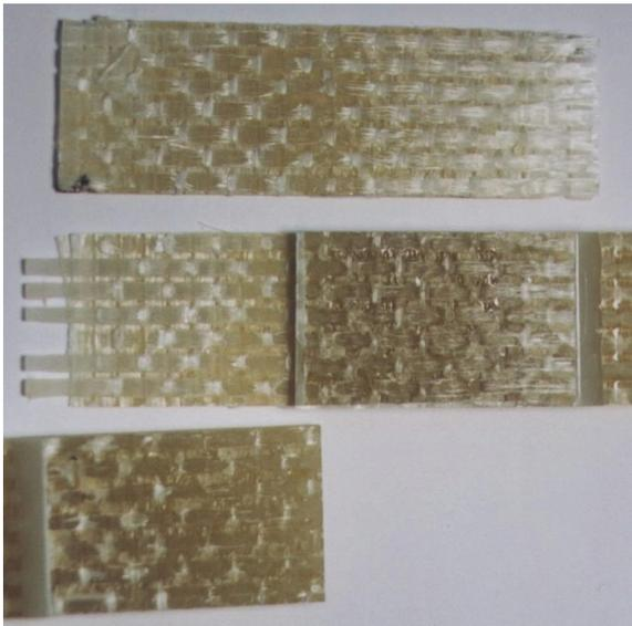
Fig. 13. Shear-type failure pattern of the DLB-7.5 joint
