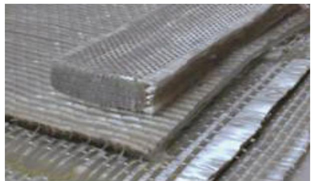
Fig. 1. Examples of 3WEAVE™ E-glass preforms
