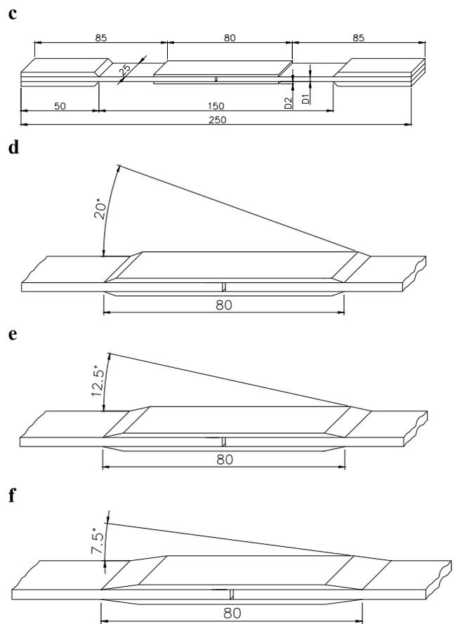
Fig. 4. Schematics of the designed and fabricated baseline flat composites (a), single-lap (using drop-off fabric) co-cured and bonded joints (b), double-lap (a.k.a. ‘double-doubler’) co-cured and bonded joints (c), and bonded tapered joints with angle 20° (d), 12.5° (e) and 7.5° (f)
