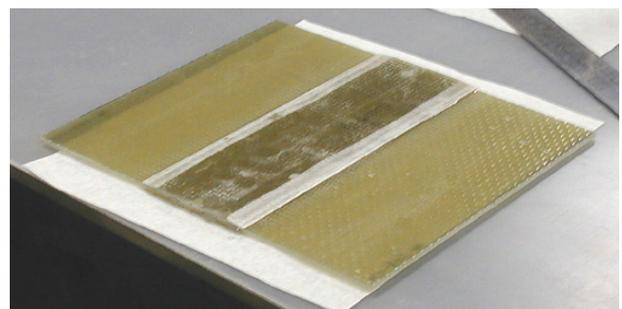
Fig. 7. Example of VARTM fabricated composite joint panel
