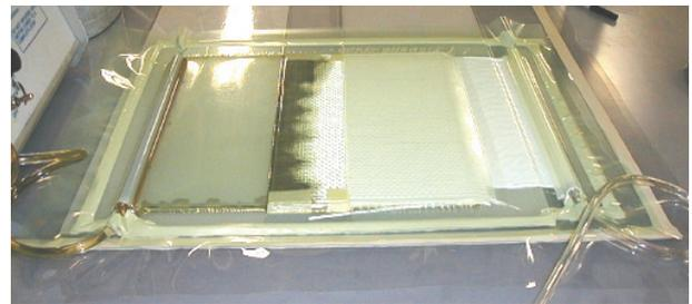
Fig. 6. Joint preform in the process of resin infusion
