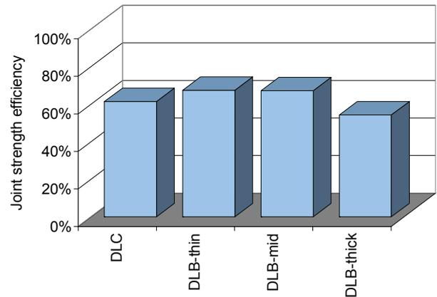
Fig. 11. JSE for the double-lap co-cured (DLC) and double-lap bonded (DLB) joints made with different outer adherend materials
