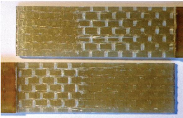
Fig. 10. Breaking pattern of the SLC joint
