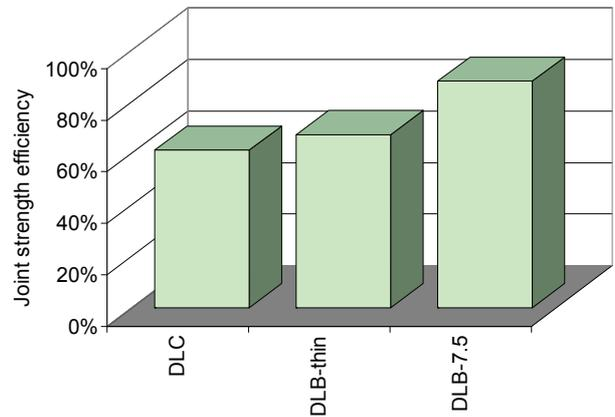
Fig. 14. Comparison of JSE values for co-cured (DLC), bonded (DLB-thin) and tapered bonded (DLB-7.5) double-lap joints
