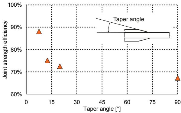
Fig. 12. Effect of taper angle on JSE of DLB joints
