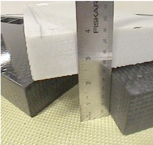
Fig. 3. Examples of composites made with single layer 3WEAVE™ glass and carbon preforms
