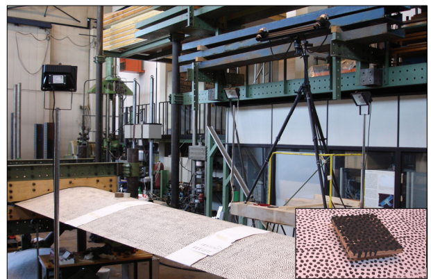
Fig. 9. Measuring pattern on the blade surface and the camera setup.
