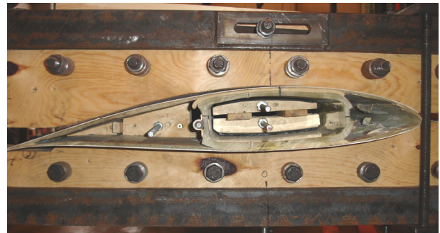
Fig. 3. Close-up picture of the tip end of the blade section, where the strengthening of cross section is visible inside the spar and trailing edge.
