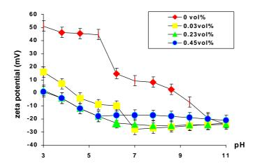
Figure 1. Zeta potential for Al<sub>2</sub>O<sub>3</sub> versus pH at different concentrations of an ammonia salt of a polymeric carboxylic acid polyelectrolyte (0.001N KNO<sub>3</sub>).
